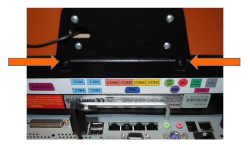
3. Plug the fingerprint reader cord into a USB port on the bottom of the station. (Any available USB port on the station can be utilized.)
