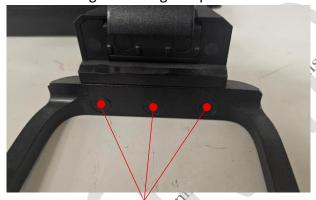
Remove the 3 rubber caps and remove the 3 screws
