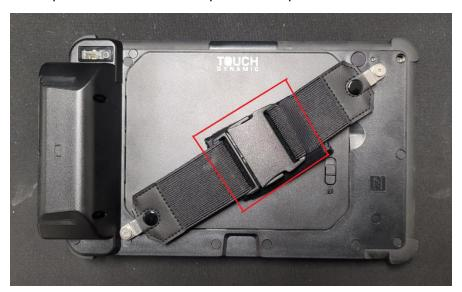
Step 5A Rotate the ends of the separated hand bands (A) away from the rear of the tablet to expose the battery door and locks.
