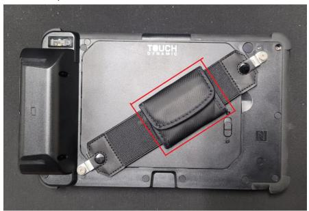
Step 4. Press the exposed tabs on the compression clip to release the band
