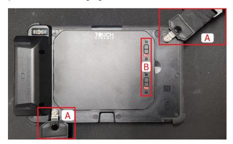
Step 6. Inserting a finger, plastic or nylon pry tool into point A, gently lift the door upwards and away to gain access to the battery compartment.
