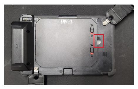
Step 7. With the battery tray door removed, firmly grip the battery pull tab, located towards the bottom of the battery and pull up and away from the rear of the tablet.
