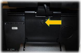
3. Make sure the cord is inserted first, down and under the counter station as you slide new pole display into place. Align the screws on the back of the station with the openings on the pole display mounting bracket.
